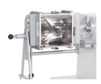
Laboratory Kneader with stainless steel kneading vessel (5 liter volume, working capacity 65%) housing two z-shaped kneading blades running at different speeds in opposing directions.
