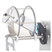
Drum Hoop Mixer with diagonal placement of the drum within the hoop, available with 5 volumes. The rotation of the hoop itself produces a uniform, three-dimensional displacement of the material to be processed and hence a tumbling mixing action.
