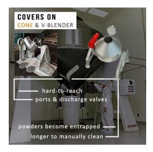
As different powders have variable viscosities and densities, they may blend well in production, but lead to issues when it comes to effective cleaning. During the blending cycle, the powders can may accumulate and amass into tight areas within the shell. Such sections which experience accumulation can be emptied during discharge, however if they are not cleared successfully, there is a heightened risk of failing to reach
