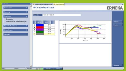
The hardness diagramms are distingushed by colour.
