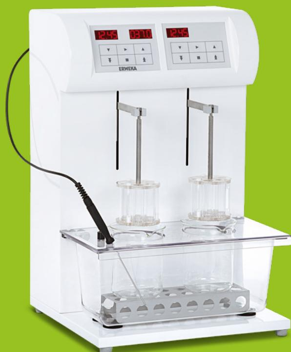
The test stations of our ZT 320 series are driven individually. Each test station is controlled by its own keypad. After programming the required test run-time, the basket rack assembly with its loaded samples is automatically lowered into the media. On completion of the preset run-time or when the stop button is pressed, the basket rack is raised from the media to prevent further disintegration of the samples (optional).
