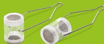
Auxiliary tubes for granule testing,
